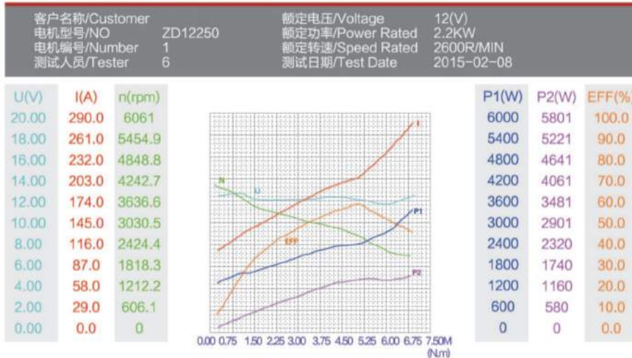
电机负载特性曲线 Motor Load Characteristic Curve
